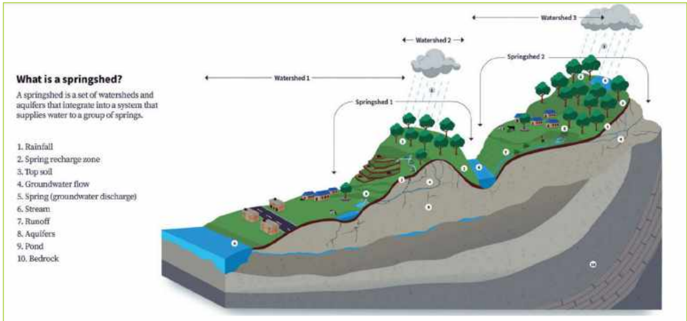
Figure 4: Schematic diagram of a springshed
